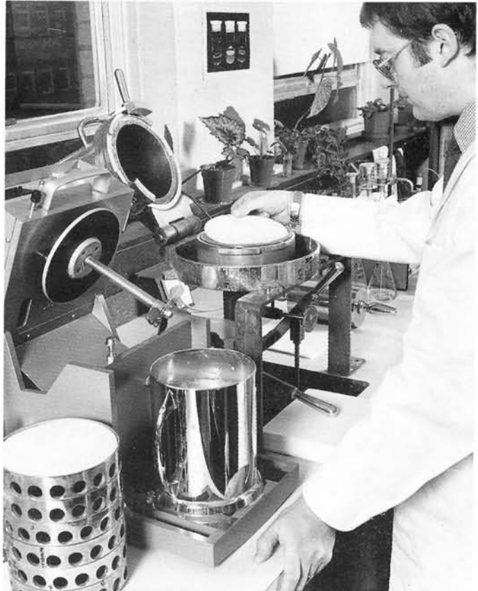
Fig 2 Preparation of wet-laid mats from fungal filaments using a British Standard Sheet Paper-making machine.
