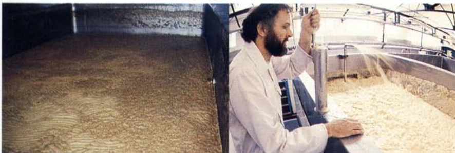
The thick yeasty foam formed on top-fermenting ale. Courtesy of Dr Malcolm Stratford (a) and Bass Breweries (b).
