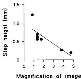
Fig. 4. Relationship between step height and the magnification of the recorded images.
