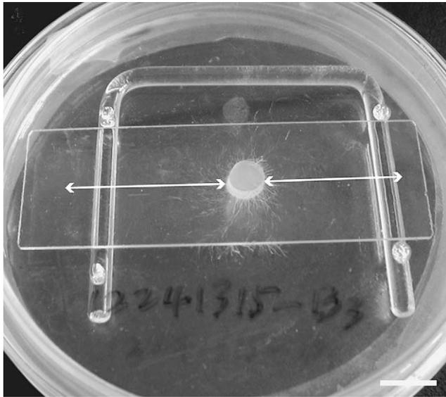
**Fig 1 – Slide culture system.** An agar-coated microscope slide is placed on a bent glass rod (diameter 4 mm) resting on moist Whatman No. 1 filter paper in a Petri dish sealed with a strip of Parafilm™. Axes for measurement of colony growth are indicated by arrowed lines. Bar = 10  $\mu\text{m}$ .
